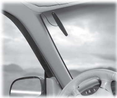
APDM5920U, vertical installation. The antenna can also be installed horizontally.
